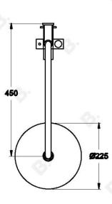
Note: bottom inlet feed requires <sup>1</sup>/<sub>2</sub>" BSP male thread in wall
