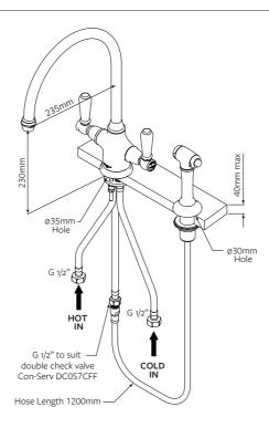
Please Note: This model does not suit incoming water pressure below tookPa or higher than 500kPa. The spray rinse model requires a minimum inlet pressure of tookPa to successfully divert the water flow from the main tap to the spray rinse. The stop cocks provided with this tap contain gauze filters. Please ensure your plumber is advised of the minimum and maximum water pressure, and to install the stop cocks as failure to do so voids the tap warranty.
