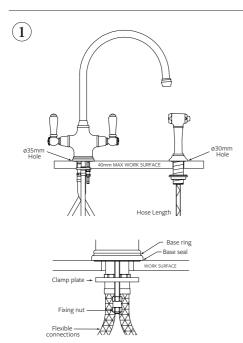
Ensure the mixer is oriented correctly, levers should rotate to point forward and the hot index should be situated on the left. Hot and cold hoses are indicated with a red or blue sticker.
