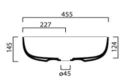
Installation Note: It is recommended that the basin be installed using a flexible sealant, epoxy type glues must not be used. To do so may void product warranty.
